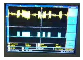
Fig. 15. Transmitted bits and the received signal
